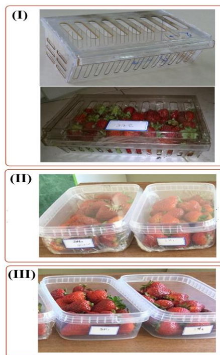
Figure 1- Packages used for packing strawberries: I. Perforated polyethylene package for pre-cooling operation, II. Perforated polyethylene package with a polymer film, III. Non-perforated polyethylene package without a polymer film
