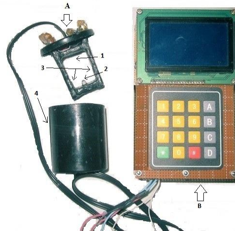
Figure 1- the scheme of the proposed system (A-measurement unit 1-photocell sensor 2- led lamp 3- electrode plates 4- plastic cup B-processing and display unit)
